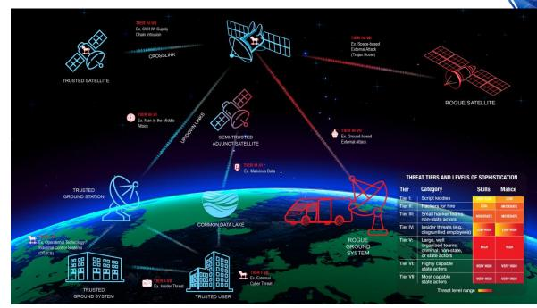
A satellite systems OV-1 illustrates segments to operations – ground, link, user, space - where threat actors could potentially impact those segments
